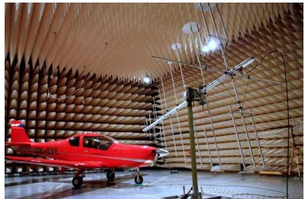
Figure 1. VUT100 Cobra in EMCC semi-anechoic chamber illuminated by a log-periodic antenna, frequency range from 20 MHz to 200 MHz
